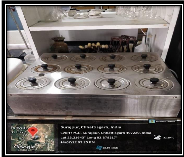
13 Rectangular water bath 8 chamber
